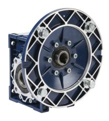
IronHorse medium-duty worm gearbox, 10:1 ratio, IEC 80B5 input, hollow, 25mm diameter output shaft, nominal 2.12hp at 1.0 SF, 664 lb-in mechanical output torque, 50mm center distance, cast aluminum housing, top, bottom and back mount.
