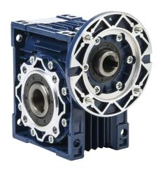
IronHorse medium-duty worm gearbox, 10:1 ratio, IEC 80B14 input, hollow, 25mm diameter output shaft, nominal 2.12hp at 1.0 SF, 664 lb-in mechanical output torque, 50mm center distance, cast aluminum housing, top, bottom and back mount.
