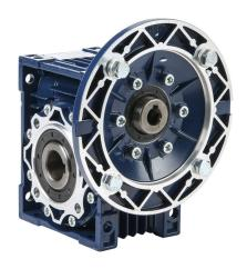
IronHorse medium-duty worm gearbox, 10:1 ratio, IEC 71B5 input, hollow, 25mm diameter output shaft, nominal 2.12hp at 1.0 SF, 664 lb-in mechanical output torque, 50mm center distance, cast aluminum housing, top, bottom and back mount.
