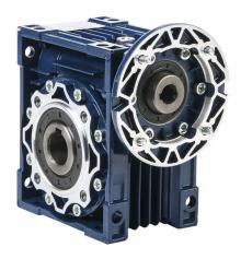
IronHorse medium-duty worm gearbox, 10:1 ratio, IEC 71B14 input, hollow, 25mm diameter output shaft, nominal 2.12hp at 1.0 SF, 664 lb-in mechanical output torque, 50mm center distance, cast aluminum housing, top, bottom and back mount.
