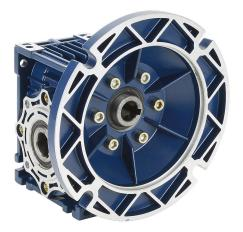
IronHorse medium-duty worm gearbox, 100:1 ratio, 56C-Face input, hollow, 0.75in diameter output shaft, nominal 0.12hp at 1.0 SF, 257 lb-in mechanical output torque, 40mm center distance, cast aluminum housing, top and bottom mount.
