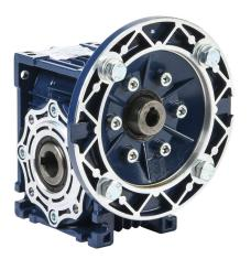
IronHorse medium-duty worm gearbox, 100:1 ratio, IEC 63B5 input, hollow, 18mm diameter output shaft, nominal 0.14hp at 1.0 SF, 244 lb-in mechanical output torque, 40mm center distance, cast aluminum housing, top, bottom and back mount.
