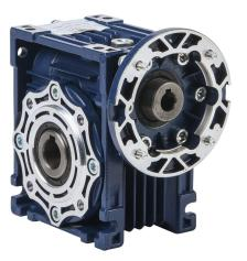
IronHorse medium-duty worm gearbox, 100:1 ratio, IEC 63B14 input, hollow, 18mm diameter output shaft, nominal 0.14hp at 1.0 SF, 244 lb-in mechanical output torque, 40mm center distance, cast aluminum housing, top, bottom and back mount.
