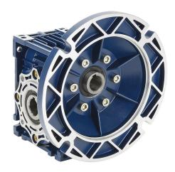
IronHorse medium-duty worm gearbox, 80:1 ratio, 56C-Face input, hollow, 0.75in diameter output shaft, nominal 0.12hp at 1.0 SF, 283 lb-in mechanical output torque, 40mm center distance, cast aluminum housing, top and bottom mount.
