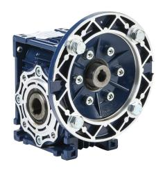
IronHorse medium-duty worm gearbox, 80:1 ratio, IEC 63B5 input, hollow, 18mm diameter output shaft, nominal 0.18hp at 1.0 SF, 277 lb-in mechanical output torque, 40mm center distance, cast aluminum housing, top, bottom and back mount.
