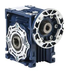
IronHorse medium-duty worm gearbox, 80:1 ratio, IEC 63B14 input, hollow, 18mm diameter output shaft, nominal 0.18hp at 1.0 SF, 277 lb-in mechanical output torque, 40mm center distance, cast aluminum housing, top, bottom and back mount.
