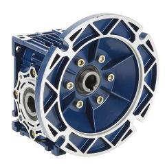
IronHorse medium-duty worm gearbox, 60:1 ratio, 56C-Face input, hollow, 0.75in diameter output shaft, nominal 0.25hp at 1.0 SF, 319 lb-in mechanical output torque, 40mm center distance, cast aluminum housing, top and bottom mount.
