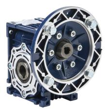
IronHorse medium-duty worm gearbox, 60:1 ratio, IEC 63B5 input, hollow, 18mm diameter output shaft, nominal 0.25hp at 1.0 SF, 319 Ib-in mechanical output torque, 40mm center distance, cast aluminum housing, top, bottom and back mount.
