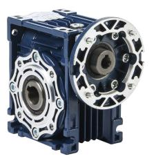
IronHorse medium-duty worm gearbox, 60:1 ratio, IEC 63B14 input, hollow, 18mm diameter output shaft, nominal 0.25hp at 1.0 SF, 319 Ib-in mechanical output torque, 40mm center distance, cast aluminum housing, top, bottom and back mount.
