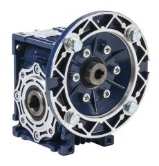
IronHorse medium-duty worm gearbox, 50:1 ratio, IEC 63B5 input, hollow, 18mm diameter output shaft, nominal 0.31hp at 1.0 SF, 353 lb-in mechanical output torque, 40mm center distance, cast aluminum housing, top, bottom and back mount.
