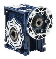
IronHorse medium-duty worm gearbox, 50:1 ratio, IEC 63B14 input, hollow, 18mm diameter output shaft, nominal 0.31hp at 1.0 SF, 353 lb-in mechanical output torque, 40mm center distance, cast aluminum housing, top, bottom and back mount.
