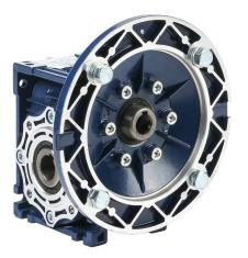
IronHorse medium-duty worm gearbox, 40:1 ratio, IEC 71B5 input, hollow, 18mm diameter output shaft, nominal 0.4hp at 1.0 SF, 378 lb-in mechanical output torque, 40mm center distance, cast aluminum housing, top, bottom and back mount.
