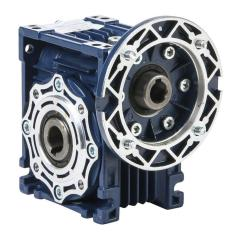
IronHorse medium-duty worm gearbox, 40:1 ratio, IEC 71B14 input, hollow, 18mm diameter output shaft, nominal 0.4hp at 1.0 SF, 378 lb-in mechanical output torque, 40mm center distance, cast aluminum housing, top, bottom and back mount.
