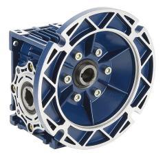
IronHorse medium-duty worm gearbox, 30:1 ratio, 56C-Face input, hollow, 0.75in diameter output shaft, nominal 0.5hp at 1.0 SF, 389 lb-in mechanical output torque, 40mm center distance, cast aluminum housing, top and bottom mount.
