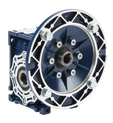
IronHorse medium-duty worm gearbox, 30:1 ratio, IEC 71B5 input, hollow, 18mm diameter output shaft, nominal 0.53hp at 1.0 SF, 403 lb-in mechanical output torque, 40mm center distance, cast aluminum housing, top, bottom and back mount.
