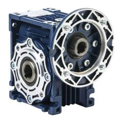
IronHorse medium-duty worm gearbox, 30:1 ratio, IEC 71B14 input, hollow, 18mm diameter output shaft, nominal 0.53hp at 1.0 SF, 403 lb-in mechanical output torque, 40mm center distance, cast aluminum housing, top, bottom and back mount.
