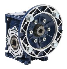
IronHorse medium-duty worm gearbox, 30:1 ratio, IEC 63B5 input, hollow, 18mm diameter output shaft, nominal 0.53hp at 1.0 SF, 403 lb-in mechanical output torque, 40mm center distance, cast aluminum housing, top, bottom and back mount.
