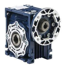
IronHorse medium-duty worm gearbox, 30:1 ratio, IEC 63B14 input, hollow, 18mm diameter output shaft, nominal 0.53hp at 1.0 SF, 403 lb-in mechanical output torque, 40mm center distance, cast aluminum housing, top, bottom and back mount.
