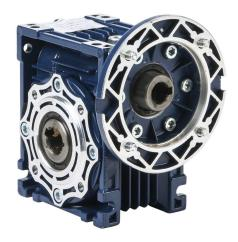
IronHorse medium-duty worm gearbox, 20:1 ratio, IEC 71B14 input, hollow, 18mm diameter output shaft, nominal 0.63hp at 1.0 SF, 361 lb-in mechanical output torque, 40mm center distance, cast aluminum housing, top, bottom and back mount.
