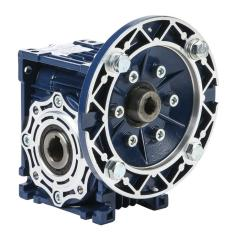
IronHorse medium-duty worm gearbox, 20:1 ratio, IEC 63B5 input, hollow, 18mm diameter output shaft, nominal 0.63hp at 1.0 SF, 361 lb-in mechanical output torque, 40mm center distance, cast aluminum housing, top, bottom and back mount.
