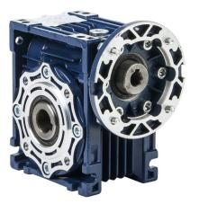
IronHorse medium-duty worm gearbox, 20:1 ratio, IEC 63B14 input, hollow, 18mm diameter output shaft, nominal 0.63hp at 1.0 SF, 361 Ib-in mechanical output torque, 40mm center distance, cast aluminum housing, top, bottom and back mount.
