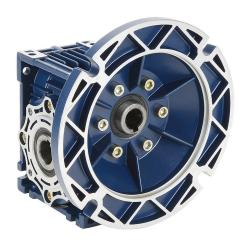
IronHorse medium-duty worm gearbox, 10:1 ratio, 56C-Face input, hollow, 0.75in diameter output shaft, nominal 1hp at 1.0 SF, 354 lb-in mechanical output torque, 40mm center distance, cast aluminum housing, top and bottom mount.
