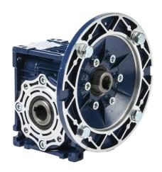
IronHorse medium-duty worm gearbox, 10:1 ratio, IEC 71B5 input, hollow, 18mm diameter output shaft, nominal 1.21hp at 1.0 SF, 370 lb-in mechanical output torque, 40mm center distance, cast aluminum housing, top, bottom and back mount.
