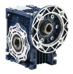
IronHorse medium-duty worm gearbox, 10:1 ratio, IEC 71B14 input, hollow, 18mm diameter output shaft, nominal 1.21hp at 1.0 SF, 370 lb-in mechanical output torque, 40mm center distance, cast aluminum housing, top, bottom and back mount.
