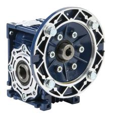
IronHorse medium-duty worm gearbox, 10:1 ratio, IEC 63B5 input, hollow, 18mm diameter output shaft, nominal 1.21hp at 1.0 SF, 370 lb-in mechanical output torque, 40mm center distance, cast aluminum housing, top, bottom and back mount.
