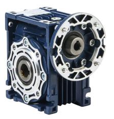
IronHorse medium-duty worm gearbox, 10:1 ratio, IEC 63B14 input, hollow, 18mm diameter output shaft, nominal 1.21hp at 1.0 SF, 370 lb-in mechanical output torque, 40mm center distance, cast aluminum housing, top, bottom and back mount.
