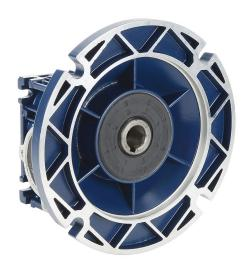
IronHorse medium-duty worm gearbox, 60:1 ratio, 56C-Face input, hollow, 0.625in diameter output shaft, nominal 0.12hp at 1.0 SF, 142 lb-in mechanical output torque, 30mm center distance, cast aluminum housing, top and bottom mount.
