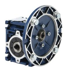
IronHorse medium-duty worm gearbox, 50:1 ratio, IEC 63B5 input, hollow, 14mm diameter output shaft, nominal 0.15hp at 1.0 SF, 151 lb-in mechanical output torque, 30mm center distance, cast aluminum housing, top, bottom and back mount.
