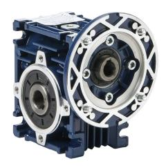
IronHorse medium-duty worm gearbox, 50:1 ratio, IEC 63B14 input, hollow, 14mm diameter output shaft, nominal 0.15hp at 1.0 SF, 151 lb-in mechanical output torque, 30mm center distance, cast aluminum housing, top, bottom and back mount.
