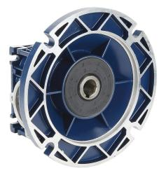
IronHorse medium-duty worm gearbox, 40:1 ratio, 56C-Face input, hollow, 0.625in diameter output shaft, nominal 0.2hp at 1.0 SF, 150 lb-in mechanical output torque, 30mm center distance, cast aluminum housing, top and bottom mount.
