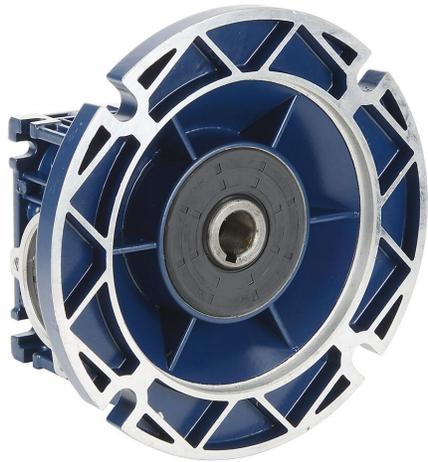
IronHorse medium-duty worm gearbox, 40:1 ratio, 56C-Face input, hollow, 0.625in diameter output shaft, nominal 0.2hp at 1.0 SF, 150 lb-in mechanical output torque, 30mm center distance, cast aluminum housing, top and bottom mount.
