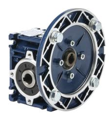
IronHorse medium-duty worm gearbox, 40:1 ratio, IEC 63B5 input, hollow, 14mm diameter output shaft, nominal 0.19hp at 1.0 SF, 160 lb-in mechanical output torque, 30mm center distance, cast aluminum housing, top, bottom and back mount.
