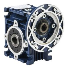
IronHorse medium-duty worm gearbox, 40:1 ratio, IEC 63B14 input, hollow, 14mm diameter output shaft, nominal 0.19hp at 1.0 SF, 160 lb-in mechanical output torque, 30mm center distance, cast aluminum housing, top, bottom and back mount.
