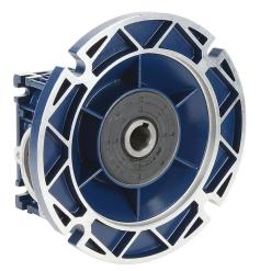
IronHorse medium-duty worm gearbox, 30:1 ratio, 56C-Face input, hollow, 0.625in diameter output shaft, nominal 0.25hp at 1.0 SF, 177 lb-in mechanical output torque, 30mm center distance, cast aluminum housing, top and bottom mount.
