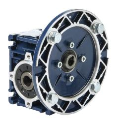
IronHorse medium-duty worm gearbox, 30:1 ratio, IEC 63B5 input, hollow, 14mm diameter output shaft, nominal 0.25hp at 1.0 SF, 177 lb-in mechanical output torque, 30mm center distance, cast aluminum housing, top, bottom and back mount.
