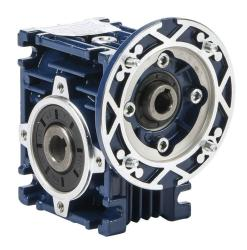
IronHorse medium-duty worm gearbox, 30:1 ratio, IEC 63B14 input, hollow, 14mm diameter output shaft, nominal 0.25hp at 1.0 SF, 177 lb-in mechanical output torque, 30mm center distance, cast aluminum housing, top, bottom and back mount.
