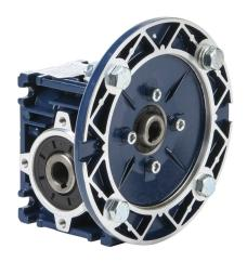
IronHorse medium-duty worm gearbox, 20:1 ratio, IEC 63B5 input, hollow, 14mm diameter output shaft, nominal 0.28hp at 1.0 SF, 151 lb-in mechanical output torque, 30mm center distance, cast aluminum housing, top, bottom and back mount.
