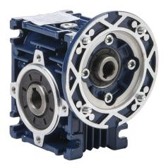
IronHorse medium-duty worm gearbox, 20:1 ratio, IEC 63B14 input, hollow, 14mm diameter output shaft, nominal 0.28hp at 1.0 SF, 151 Ib-in mechanical output torque, 30mm center distance, cast aluminum housing, top, bottom and back mount.
