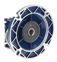
IronHorse medium-duty worm gearbox, 10:1 ratio, 56C-Face input, hollow, 0.625in diameter output shaft, nominal 0.5hp at 1.0 SF, 150 lb-in mechanical output torque, 30mm center distance, cast aluminum housing, top and bottom mount.
