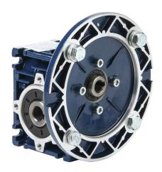
IronHorse medium-duty worm gearbox, 10:1 ratio, IEC 63B5 input, hollow, 14mm diameter output shaft, nominal 0.54hp at 1.0 SF, 160 lb-in mechanical output torque, 30mm center distance, cast aluminum housing, top, bottom and back mount.
