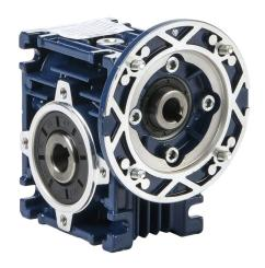
IronHorse medium-duty worm gearbox, 10:1 ratio, IEC 63B14 input, hollow, 14mm diameter output shaft, nominal 0.54hp at 1.0 SF, 160 lb-in mechanical output torque, 30mm center distance, cast aluminum housing, top, bottom and back mount.
