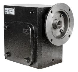
IronHorse heavy-duty worm gearbox, 60:1 ratio, 145TC-Face input, right hand, 1.375in diameter output shaft, nominal 2hp at 1.0 SF, 3127 lb-in mechanical output torque, 3-1/4in center distance, cast iron housing, tapped-base mount.
