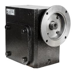
IronHorse heavy-duty worm gearbox, 60:1 ratio, 56C-Face input, right hand, 1.375in diameter output shaft, nominal 2hp at 1.0 SF, 3127 lb-in mechanical output torque, 3-1/4in center distance, cast iron housing, tapped-base mount.
