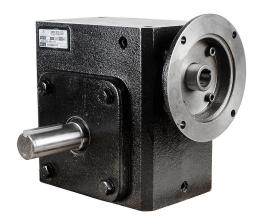
IronHorse heavy-duty worm gearbox, 60:1 ratio, 145TC-Face input, left hand, 1.375in diameter output shaft, nominal 2hp at 1.0 SF, 3127 lb-in mechanical output torque, 3-1/4in center distance, cast iron housing, tapped-base mount.
