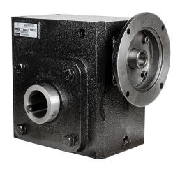
IronHorse heavy-duty worm gearbox, 60:1 ratio, 145TC-Face input, hollow, 1.937in diameter output shaft, nominal 2hp at 1.0 SF, 3127 lb-in mechanical output torque, 3-1/4in center distance, cast iron housing, tapped-base mount.
