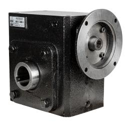
IronHorse heavy-duty worm gearbox, 60:1 ratio, 56C-Face input, hollow, 1.937in diameter output shaft, nominal 2hp at 1.0 SF, 3127 lb-in mechanical output torque, 3-1/4in center distance, cast iron housing, tapped-base mount.
