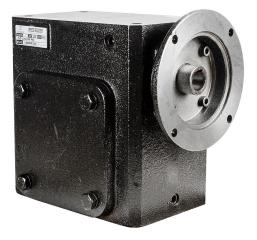
IronHorse heavy-duty worm gearbox, 40:1 ratio, 145TC-Face input, right hand, 1.375in diameter output shaft, nominal 2hp at 1.0 SF, 3692 lb-in mechanical output torque, 3-1/4in center distance, cast iron housing, tapped-base mount.
